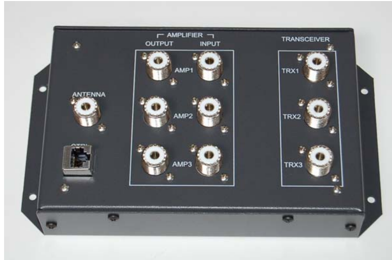
The completed StationPro RF relay unit
