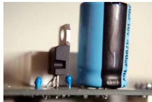
The 7805 voltage regulator is vertically mounted and sits about 1/4" above the circuit board.
