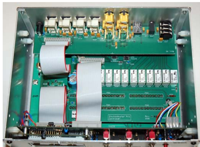
Interior view of the completed SP-II Control Unit
