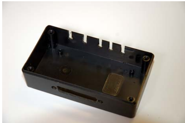
Completed enclosure with five slots, which hold a total of ten cables (for a Yaesu FT-2000 transceiver)
