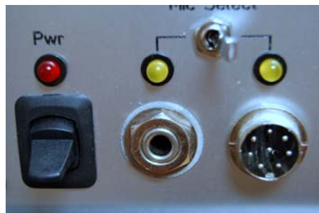
The Collins-type 3/16” mic jack is insulated from the front panel using homemade fiberglass washers on the front and back sides of the panel
