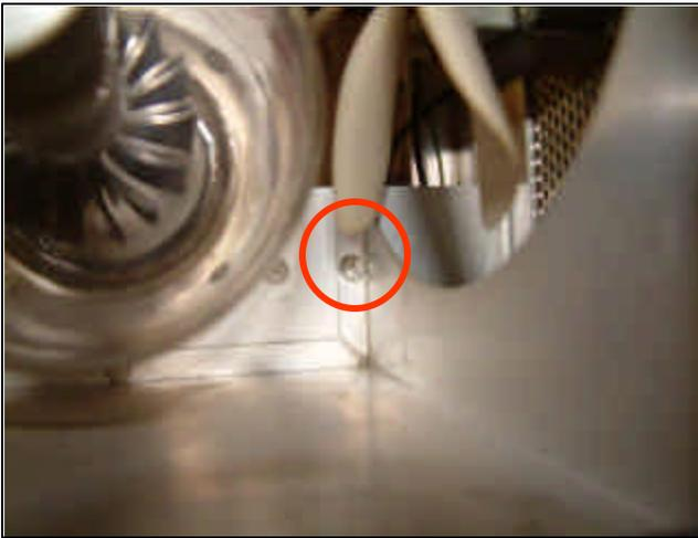
Locate the screw in the tube compartment that is held in place by this nut (it is near the corner of this compartment at the rear). Loosen this screw and remove the nut and lock washer from the underside of the chassis.
