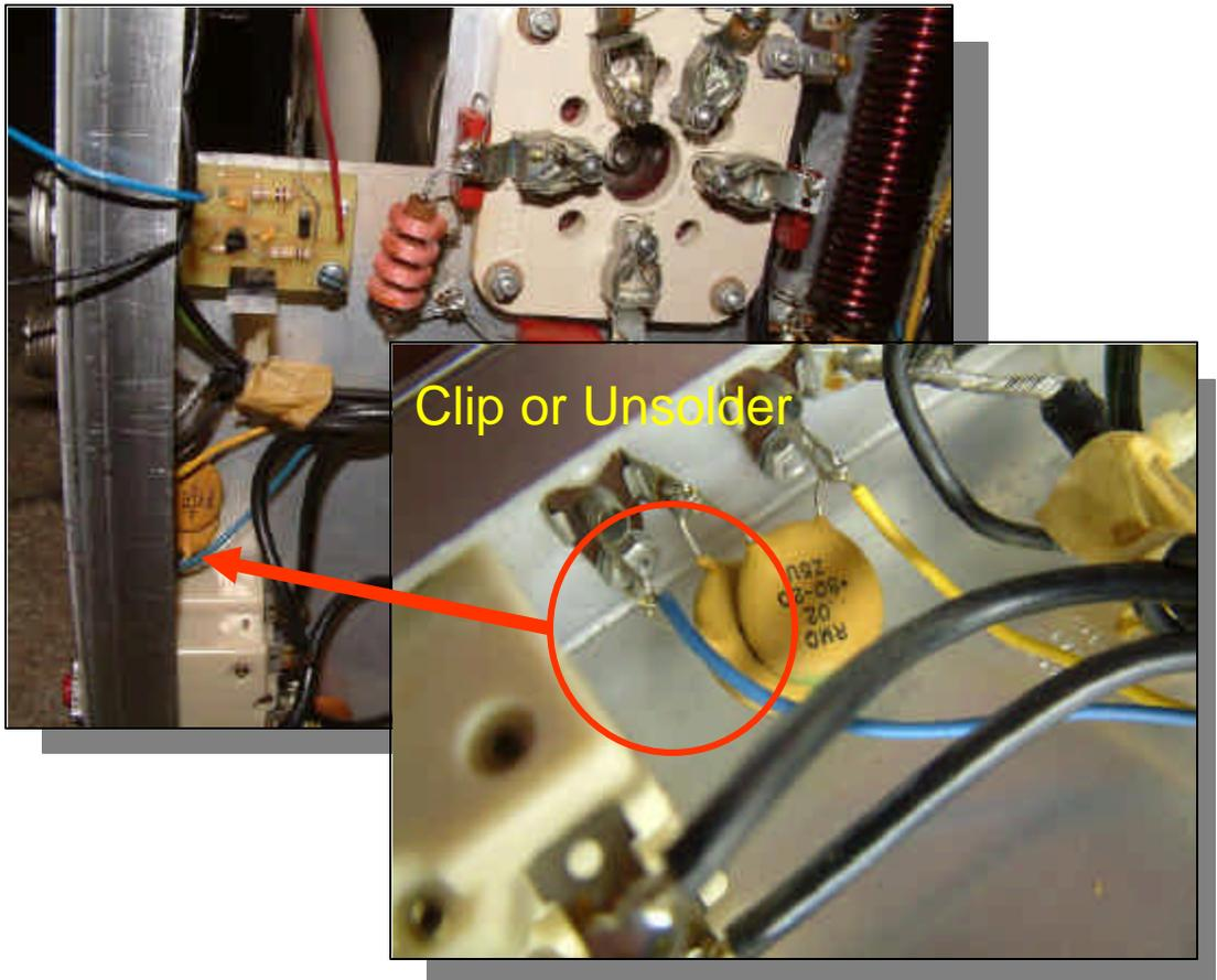
Strip about ¼" of insulation from this wire. Pass the wire under the
