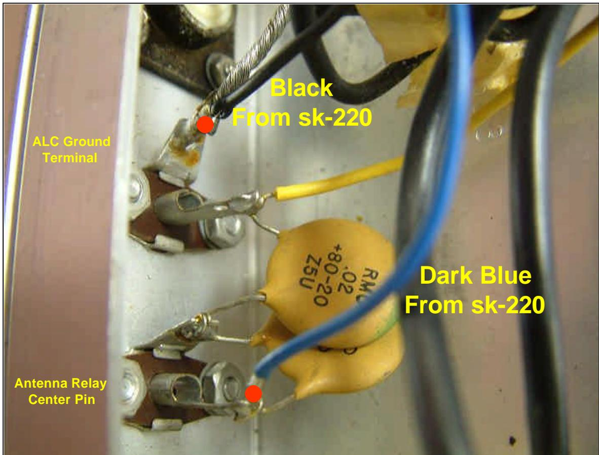
Pass the **DARK BLUE** wire from the SK-220 circuit board under the wire harness and solder it to the center pin of the antenna relay jack on the rear panel.
