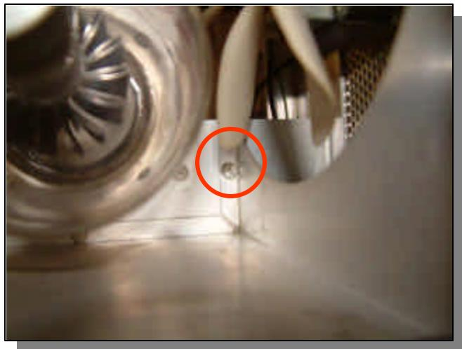
Locate the screw in the tube compartment that is held in place by this nut (it is near the corner of this compartment at the rear). Loosen this screw and remove the nut and lock washer from the underside of the chassis.
