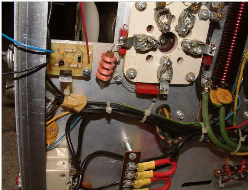
Pass the **BLACK** wire from the SK-220 circuit board under the wire harness and solder it to the ground lug on the ALC jack on the rear panel.
