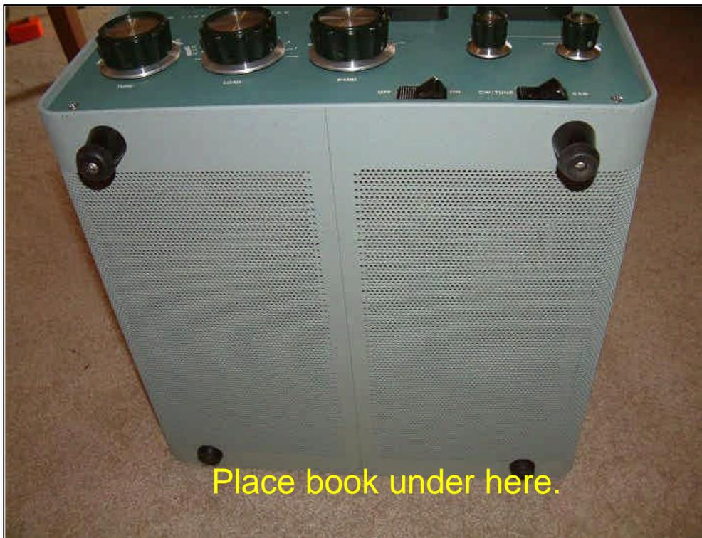
Lift the case up and remove it from the amplifier.
